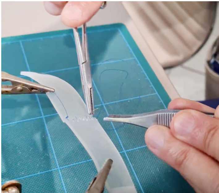
Figure 2: Uniaxial tensile test performed on a 3D printed sample sutured by an expert surgeon in order to mimic the surgical suture on a medium caliber arterial vessel.
