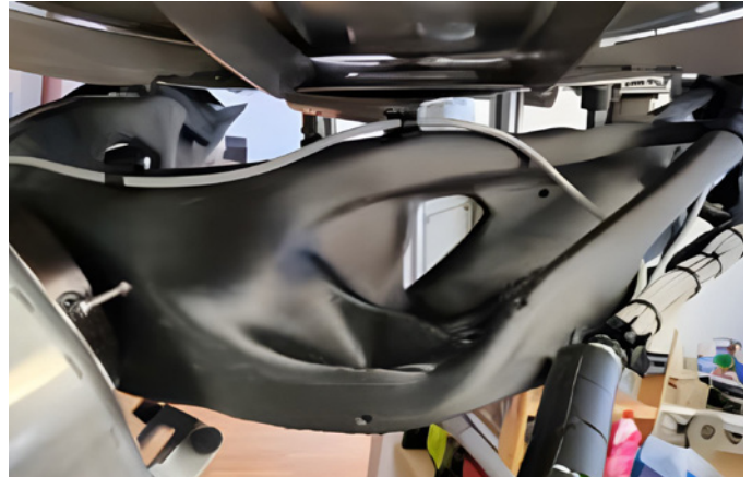
The 3D printed Nylon 12CF mount (black) is shown installed on the antenna assembly.
